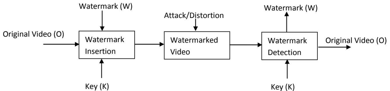
**Figure 2: Block diagram of a video watermarking system**
