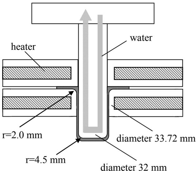
Fig. 9. Schematic illustration of experimental apparatus for hot deep drawing. Puch speed was 1.2 mm/s. Heating temperature was 250°C. Lubricant was Teflon sheet
