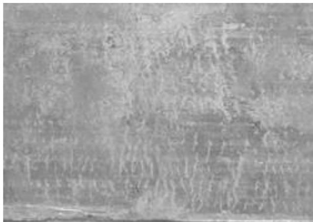
Fig. 11. AZ91 as cast strip. Roll speed was 90 m/min. Thickness was 1.5 mm
