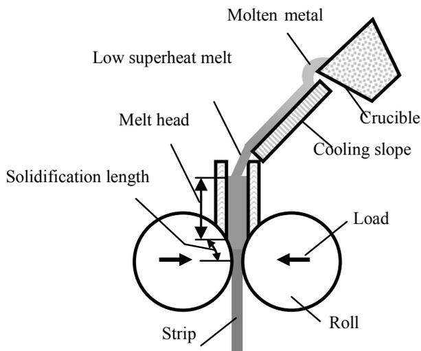
Fig.1. Schematic illustration of a high speed twin roll caster
