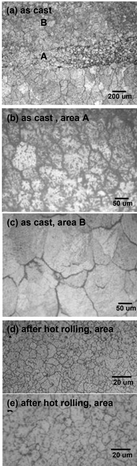
Fig. 6. Microstructure of as cast and hot rolled AZ31 strip. Pass schedule of hot rolling is as below. 1st pass: 350 °C-1h from 1.7 mm to 1.0 mm, 2nd pass: 350 °C-0s from 1.0 mm to 0.7 mm, 3rd pass: 350 °C-0s from 0.7 mm to 0.5 mm
