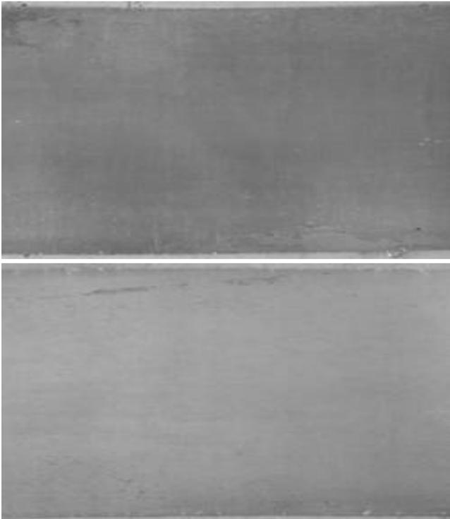
Fig. 12. Hot rolled AM60 and AZ91 sheet. Holding temperature, holding time and reduction of each pass was as below, 1st pass: 420 °C-1h from 1.5 mm to 1.2 mm, 2nd pass: 420 °C-0s from 1.2 mm to 0.9 mm, 3rd pass: 420 °C-0s from 0.9 mm to 0.7 mm, 4th pass: 420 °C-0s from 0.7 mm to 0.5 mm
