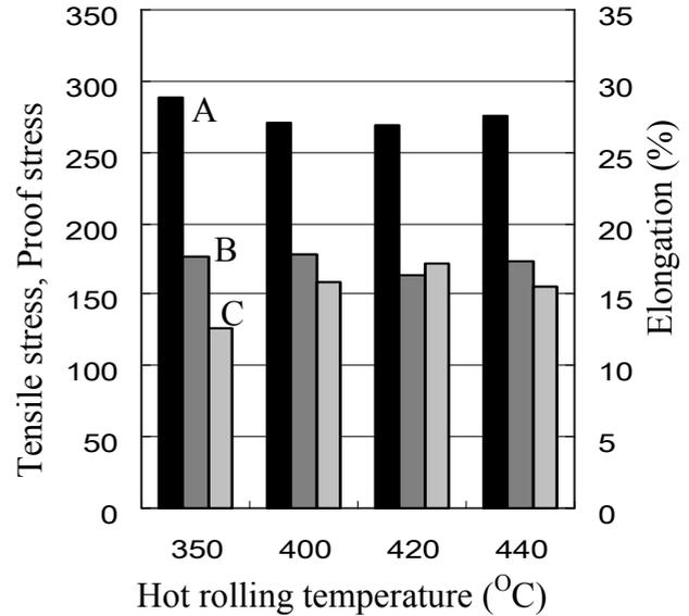
Fig. 7. Influence of temperature of hot rolling on tension test of AZ31 sheet. Pass schedule of hot rolling and annealing is as below. 1st pass: holding-1h from 1.7 mm to 1.0 mm, 2nd pass: holding-0s from 1.0 mm to 0.7 mm, 3rd pass: holding-0s from 0.7 mm to 0.5 mm, annealing: 300 °C-1h. Specimen is as below. Gage length: 20 mm, width 10 mm, thickness: 0.5 mm. A: tensile stress, B: proof stress, C: elongation
