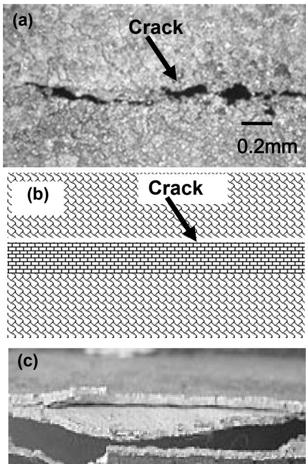
Fig. 14. Center line crack of as cast strip. (a) shows the photograph by optical microscope, (b) shows schematic illustration of the (a), and (c) shows cross section of the broken strip after continuous bending.
