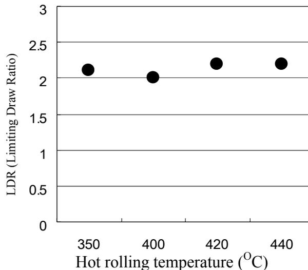
Fig. 10. Influence of temperature of hot rooling on LDR (Limiting Draw Ratio)of AZ31 sheet at hot deep drowing. Work temperature was 250 °C. Puch speed was 1.2 mm/s. Lubricant was Teflon sheet. Pass schedule of hot rolling and annealing is as below. 1st pass: holding-1h from 1.7 mm to 1.0 mm, 2nd pass: holding-0s from 1.0 mm to 0.7 mm, 3rd pass: holding-0s from 0.7 mm to 0.5mm, annealing: 300°C-1h
