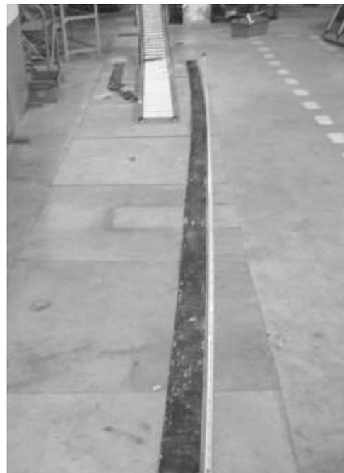
Fig. 2. An as cast strip of AZ31. Length was about 5 mm. Roll speed was 150 m/min. Width was 100 mm
