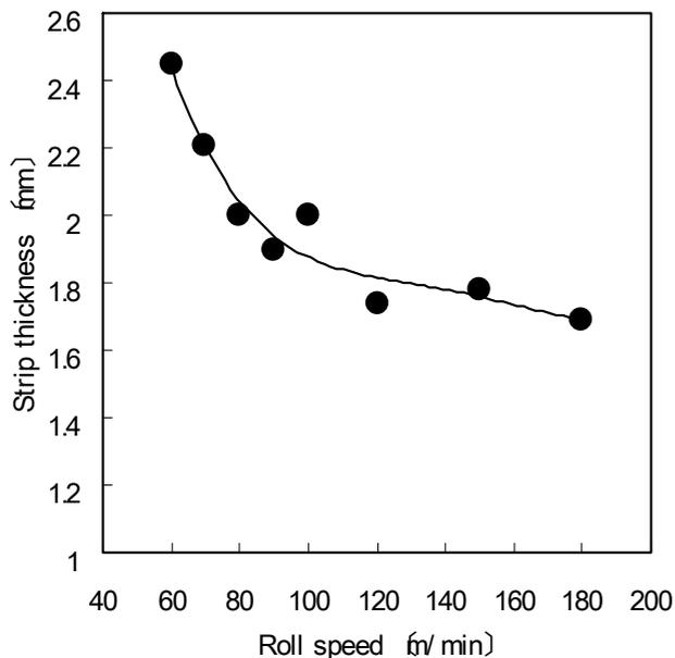
Fig. 4. Relationship between roll speed and thickness of AZ31 as cast strip. Contact length was 80 mm
