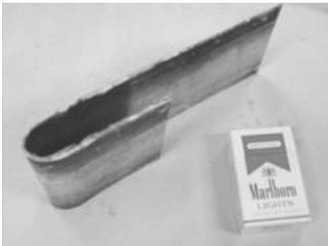
Fig. 3. 180 degrees bending of as cast AZ31 strip at radius curvature of 15 mm
