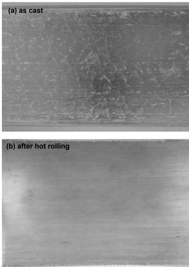
Fig. 5. As cast and hot rolled AZ31 strip. Pass schedule of hot rolling is as below. 1st pass: 350 °C-1h from 1.7 mm to 1.0 mm, 2nd pass: 350 °C-0s from 1.0 mm to 0.7 mm, 3rd pass: 350 °C-0s from 0.7 mm to 0.5mm
