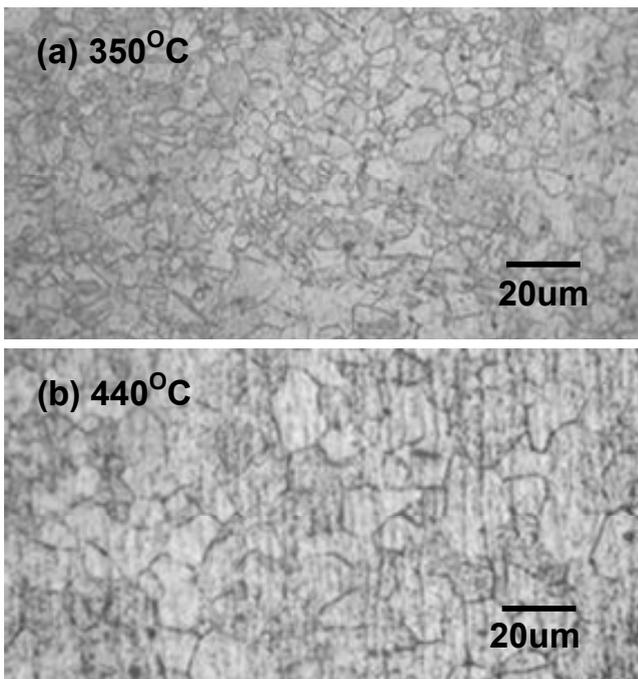
Fig. 8. Influence of temperature of hot rooling on microstructure of AZ31 sheet. Pass schedule of hot rolling and annealing is as below. 1st pass: holding-1h from 1.7 mm to 1.0 mm, 2nd pass: holding-0s from 1.0 mm to 0.7 mm, 3rd pass: holding-0s from 0.7 mm to 0.5mm, annealing: 300°C-1h
