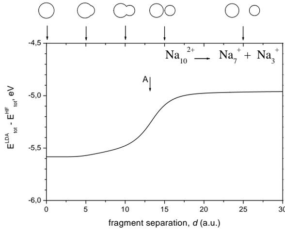
FIG. 7: Difference between the LDA and HF total energies as a function of fragments separation distance for the fission channel  $Na_{10}^{2+} \rightarrow Na_7^+ + Na_3^+$ . The evolution of the cluster shape during the fission process is shown on top of the figure. Vertical arrow A corresponds to the scission point.
