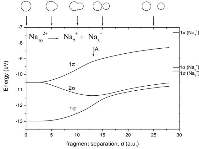
FIG. 1: Hartree-Fock single electron energy levels for the asymmetric fission channel  $Na_{10}^{2+} \rightarrow Na_7^+ + Na_3^+$  as a function of fragments separation distance  $d$ , when both the parent and daughter clusters are spherical ( $\delta_0 = \delta_1 = \delta_2 = 0$ ). The evolution of the cluster shape during the fission process is shown on top of the figure. Horizontal lines on the right hand side of the figure mark the Hartree-Fock energy levels for the free daughter fragments.
