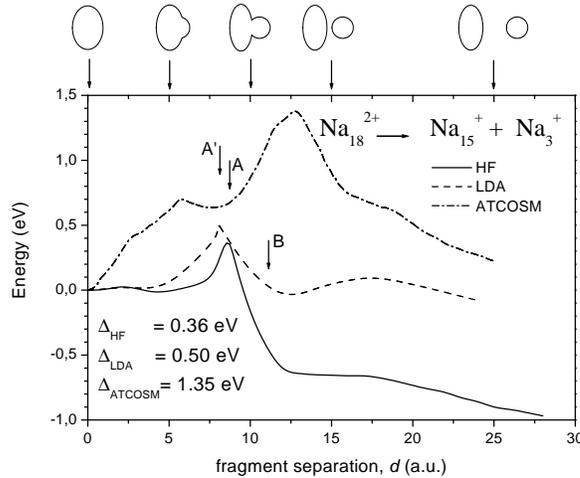
FIG. 5: The same as figure 4, but for the asymmetric channel  $Na_{18}^{2+} \rightarrow Na_{15}^+ + Na_3^+$
