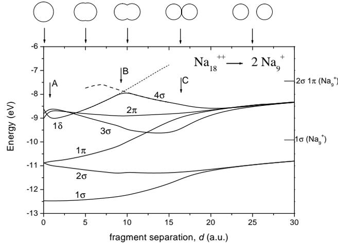
FIG. 3: The same as figure 1 but for symmetric fission channel  $\text{Na}_{18}^{2+} \rightarrow 2\text{Na}_9^{+}$ . Lowest unoccupied states are shown by dashed ( $4\sigma$ ) and short dashed ( $2\pi$ ) lines.
