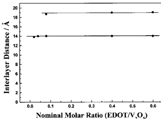
FIGURE 4 Evolution of interlayer distance upon increasing nominal molar ratio of EDOT to  $V_2O_5$ .
