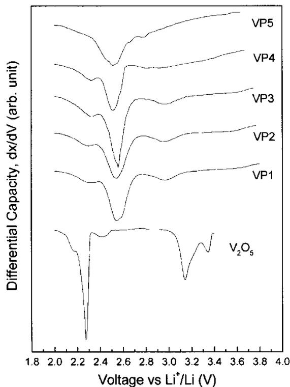
FIGURE 7 The first differential capacity profiles of the first discharges of the pristine  $V_2O_5$  and hybrids.
