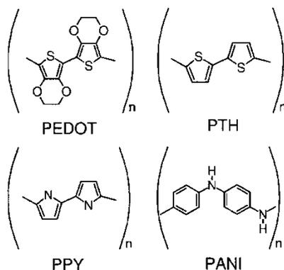
FIGURE 1 Chemical structure of some selected conductive polymers: PEDOT (poly(3,4-ethylene dioxithiophene)), PTH (polythiophene), PPY (polypyrrole) and PANI (polyaniline).
