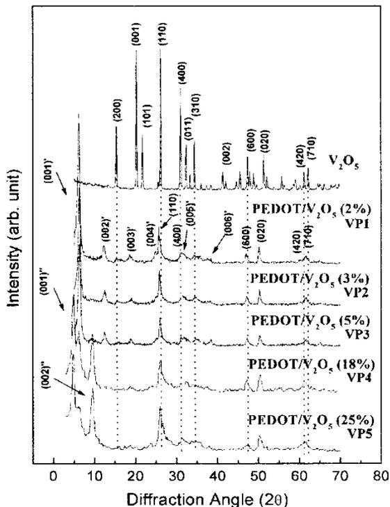
FIGURE 3 Powder X-ray diffraction patterns of pristine  $V_2O_5$ , VP1, VP2, VP3, VP4 and VP5.
