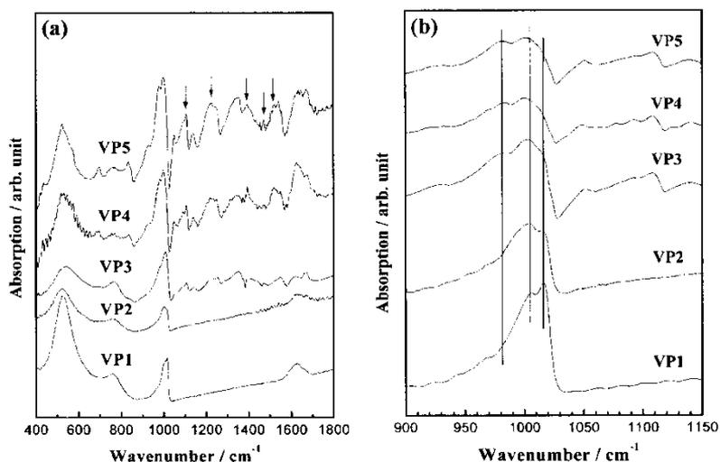
FIGURE 5 Infrared spectra for VP1, VP2, VP3, VP4 and VP5 in the range of (a) 400–1800 cm<sup>-1</sup> and (b) 900–1150 cm<sup>-1</sup> (enlargement). The samples were diluted with KBr and pressed into a pellet. Some important peaks from the polymer are marked with arrows.
