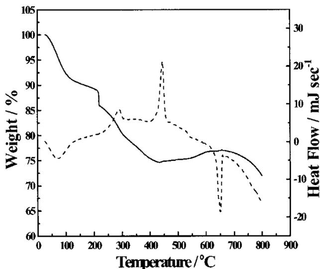
FIGURE 2 Thermogravimetry (solid line) and differential scanning calorimetry (dashed line) curves for VP3 sample as a representative.
