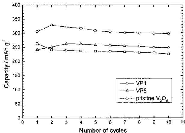
FIGURE 8 Evolution of discharge capacity with the number of cycles for pristine  $V_2O_5$ , VP1 and VP5. The data were obtained at a current density of 15 mA/g. The potential range was set to 2.0–4.2 V vs. Li for  $V_2O_5$ , and to 2.0–4.4 V for VP1 and VP5.
