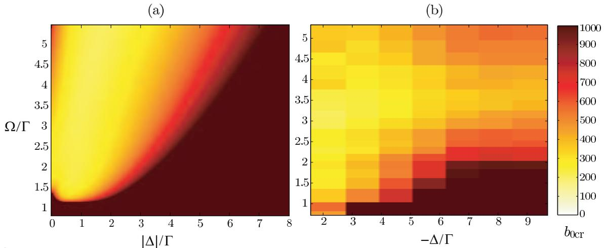
**Figure 9.** Threshold of random lasing based on Mollow gain (left) and Raman gain (right) for each pair of pumping parameters  $\Delta$  (detuning) and  $\Omega$  (Rabi frequency). We use the theoretical knowledge of the atomic polarizability (11) for Mollow gain whereas the prediction for Raman gain is based on experimental spectra (see text). In both cases, we obtain a minimum optical thickness of about 200.
