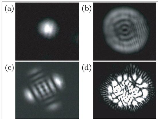
**Figure 1.** Transverse modes of cold-atom lasers. (a) Gaussian  $TEM_{00}$  mode, obtained by inserting a small diaphragm in the cavity. Typical modes of: (b) the Mollow laser, (c) the Raman laser, and (d) the four-wave mixing laser respectively.
