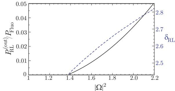
**Figure 10.** Continuous line: Emitted random laser power normalized to the pump fluorescence power, as a function of the pump intensity. Dashed line: Normalized laser detuning  $\delta_{\text{RL}}$ . The random medium is a spherical cloud of two level atoms with an on-resonance optical-thickness  $b_0 = 600$ .
