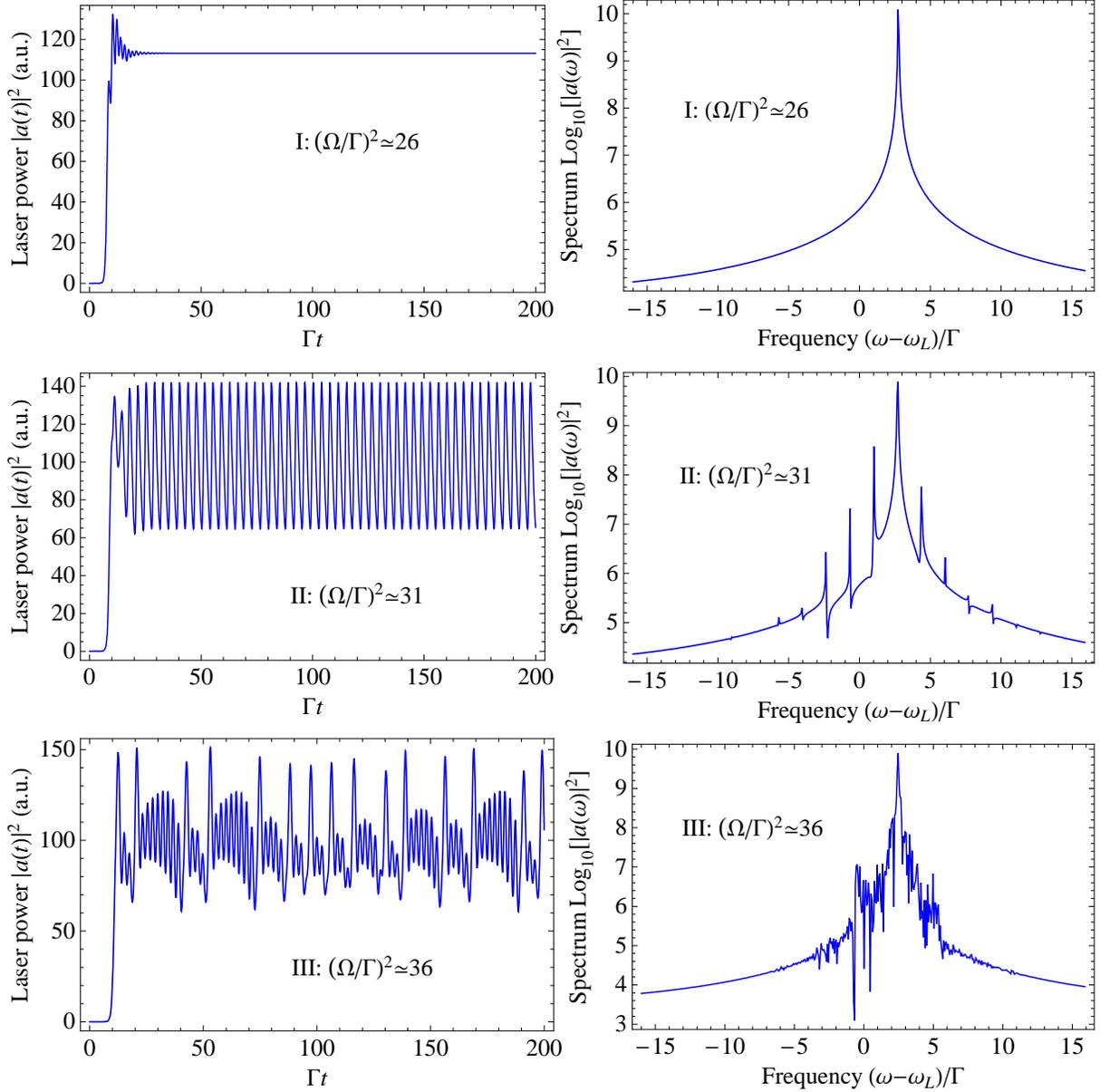
**Figure 8.** Laser power versus time (left) and corresponding spectra (right) for the three different regimes of lasing: I – single-mode lasing, II – multi-mode lasing, and III – chaotic behaviour. The spectra are calculated in the stationary regime  $\Gamma t > 100$ . The parameters used in the calculation are the same as in figure 7.
