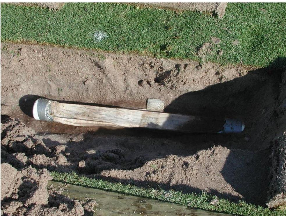
**Picture 3.** Lysimeter collection containers extending beyond the lower end of the instrumented turfgrass plot (summer 2004).
