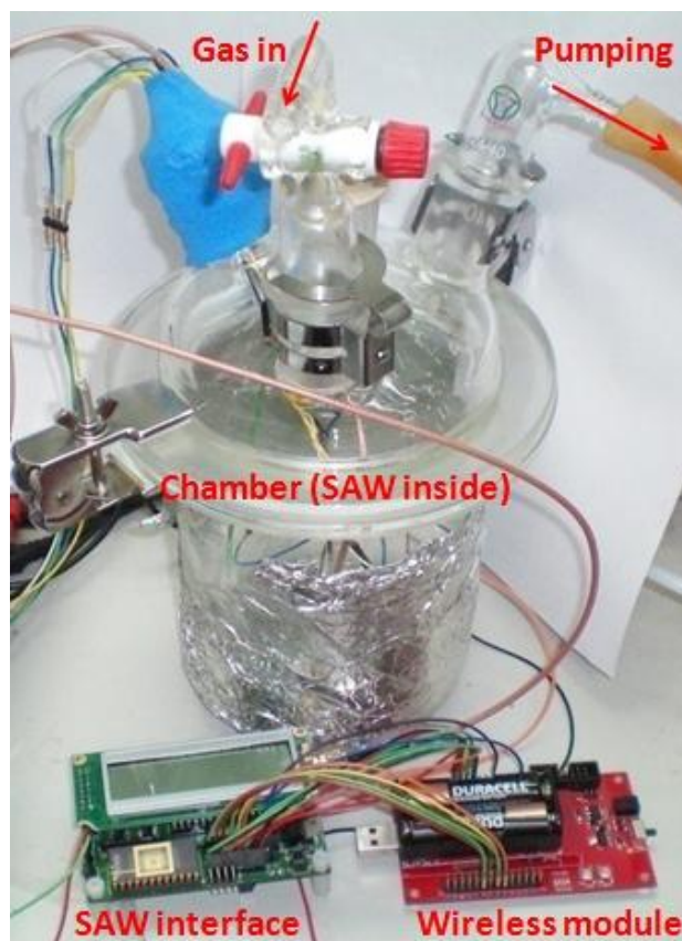
Figure 10. Test setup of the sensor node.
