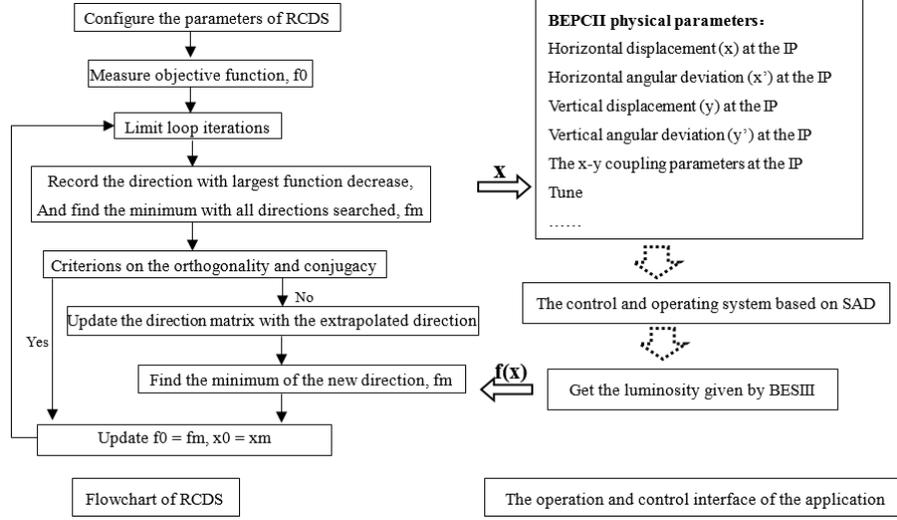
Fig. 3. Flowchart of RCDS for online optimization of the luminosity of BEPCII and the data stream between the RCDS method and operation of BEPCII.
