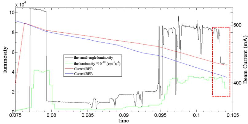
Fig. 6. (color online) The change process of the luminosity given by BESIII
