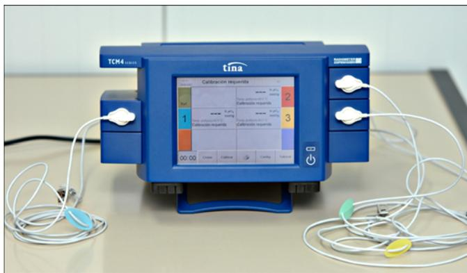
**Figure 1.** System analysis of transcutaneous oxygen pressure with TCM400 monitor (Radiometer Medical ApS; Copenhagen, Denmark).
