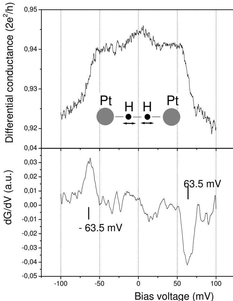
FIG. 2: Differential conductance (top) and its derivative (bottom) for a Pt/H<sub>2</sub> contact taken at a conductance plateau close to  $1 G_0$ . The differential conductance is recorded by a lock-in amplifier using a modulation amplitude between 0.88 and 1.5 mV<sub>rms</sub> at 7 kHz and a time constant of 10 ms, and the derivative is numerically calculated. A full spectrum is recorded in 10 s.
