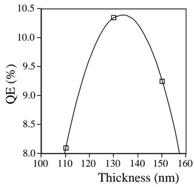
Figure 2: Quantum efficiencies versus the thickness of the CsI photocathode.
