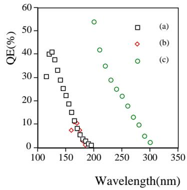
Figure 3: Quantum efficiencies of optimized photocathodes: (a) CsI with a  $\text{MgF}_2$  window, (b) CsI with a quartz window, and (c) CsTe with a quartz window.
