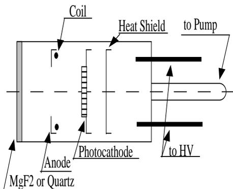
Figure 1: Cross-sectional view of the test phototube. The cathode was made of Al-plated Ni-electrode. The photocathodes were plated on it.
