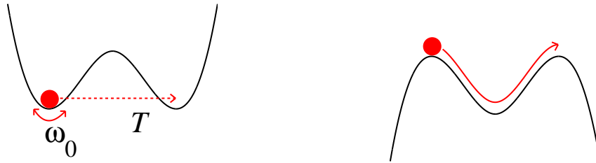
FIGURE 14. Tunneling of a particle in a double-well potential (left); in imaginary time, this tunneling event (instanton) is described by the dynamics in the inverted potential (right).
