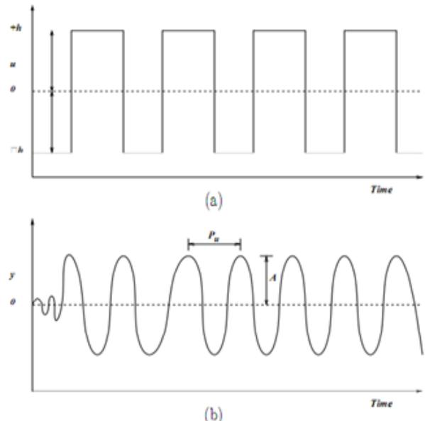
Figure 10. The effect of fluctuations on / off a relay.
