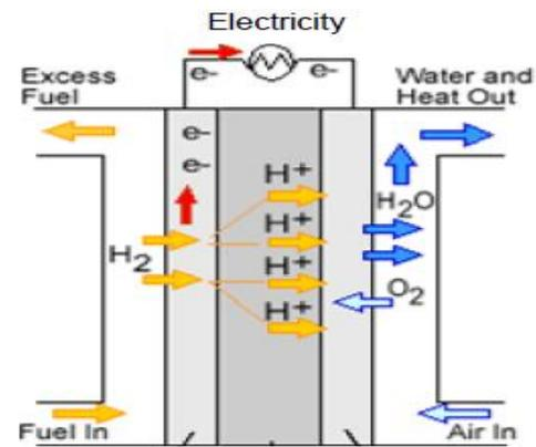
Figure 13. Proton exchange membrane fuel cell
