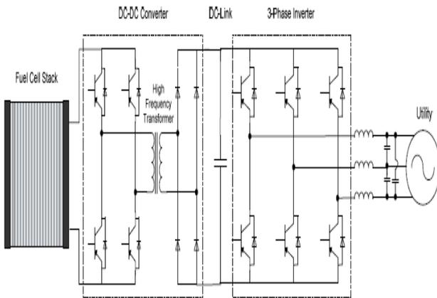
Figure 16. Cascaded DC-DC and DC-AC converter topology (DC-link)
