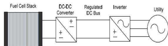
Figure 15. Fuel cell system configuration with cascaded DC-DC and DC-AC converters.
