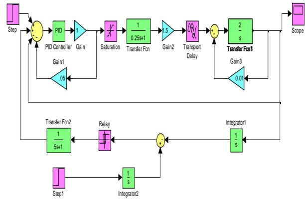
Figure 3. Dynamical model of synchronizer
