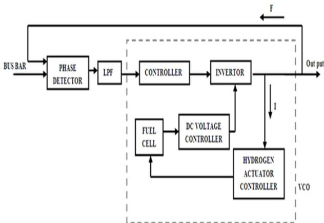
Figure 2. Block diagram of synchronizer fuel cell
