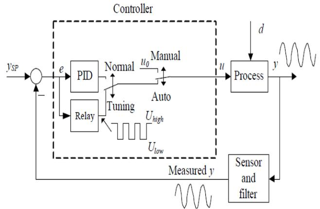
Figure 9. PID autotuning Structures based on control (on / off) of Relay
