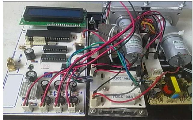
Figure 17. Synchronizer digital devices for both motors
