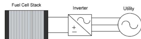
Figure 14. Fuel cell system configuration with a single inverter
