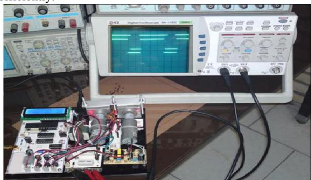
Figure 23 digital outputs Synchronizer practical test
