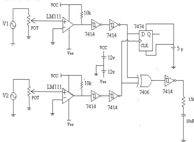
Figure 11. Synchronizer circuit Schematic
