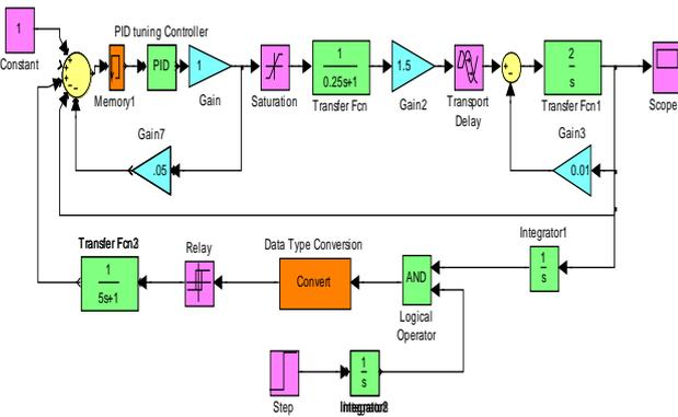
Figure 7. Synchronizer dynamic model of the ZVS
