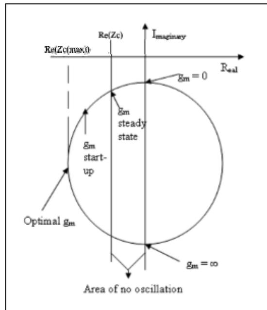
Figure 3. Complex plane representation of the negative resistance.
