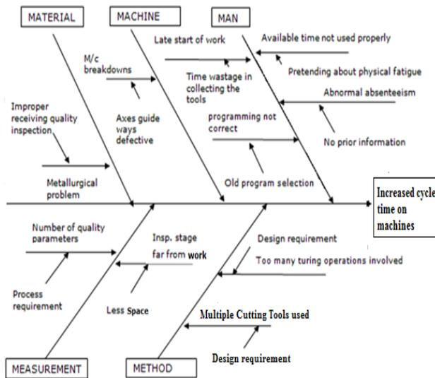
Fig. 3 Cause and Effect Diagram
