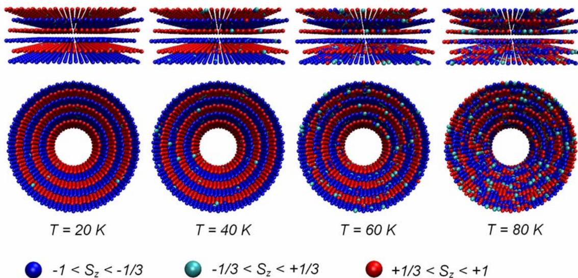
**Figure 3.** Snapshots of spin ordering in the bulk  $\text{NiCl}_2$  and six-walled  $\text{NiCl}_2$  nanotube  $(20,20)@(26,26)@(32,32)@(38,38)@(44,44)@(50,50)$  at different temperatures.
