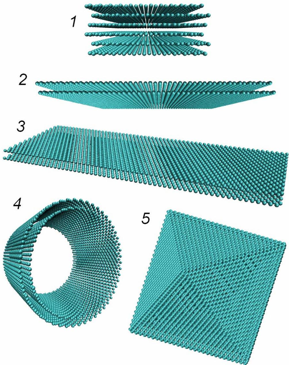
**Figure 1.** Structures of the bulk  $\text{NiCl}_2$  (1), infinite  $\text{NiCl}_2$  bilayer (2), one-dimensional (12,12)  $\text{NiCl}_2$  nanostripe (3), double-walled (44,44)@(50,50)  $\text{NiCl}_2$  nanotube (4) and fullerene  $(\text{NiCl}_2)_{2304} @ (\text{NiCl}_2)_{3136}$  (5). Nickel atoms are only shown.
