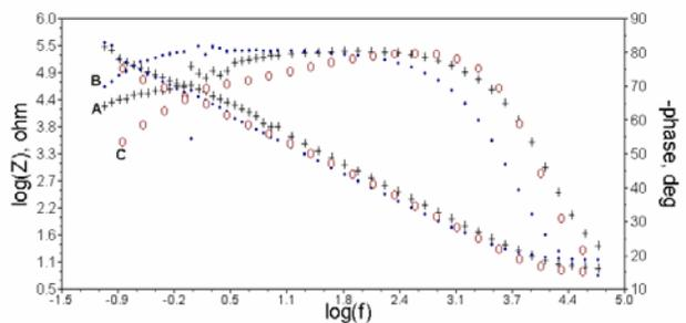
Fig. 3. Bode plots of impedance spectra for electropolished (A) sterilized (B) and thermally passivated (C) samples
