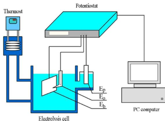
Fig. 1. Diagram of the corrosion resistance set
