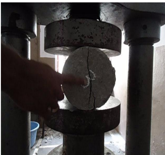
Fig. 3 Testing of Cylinder during split tensile strength test
