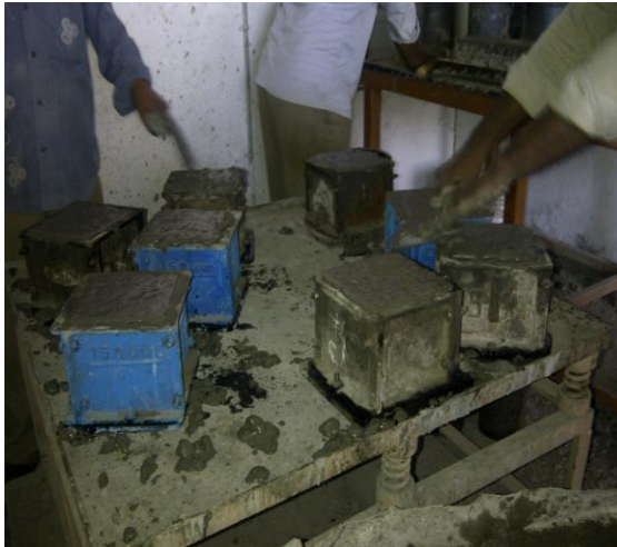
Fig. 1 Cubes on Vibrating table during Compaction
