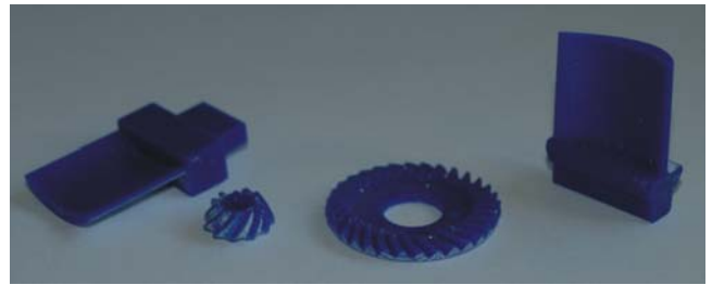
Fig. 5. Wax models made by means of CPX 3000 device
