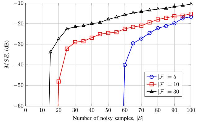
Fig. 3: Behavior of Mean Squared Error versus number of noisy samples, for different signal bandwidths.
