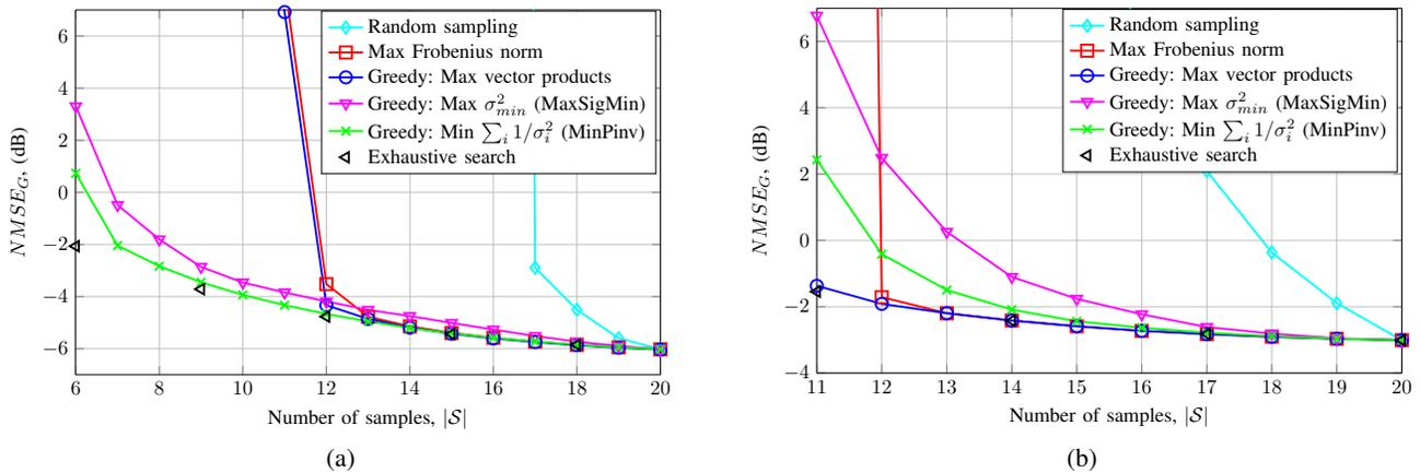
Fig. 4: Behavior of Mean Squared Error versus number of samples, for different sampling strategies for a scale-free topology. (a) for the case of  $|\mathcal{F}| = 5$ , whereas (b) for the case  $|\mathcal{F}| = 10$ .
